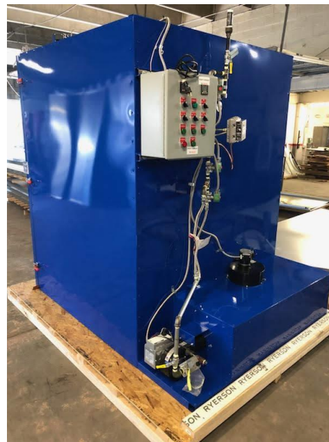
Figure 2: EPTEX Gas Oven PID and heater
